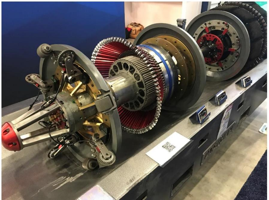
*A BIG pipeline inspection gauge (“PIG”) used to inspect the inside of pipelines.*
